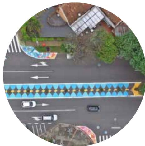
An interim median barrier can trial the effect on the traffic for a longer period of time.
