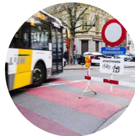
The interim installation allows the impact on the network to be tested over a longer period of time, to monitor changes in behaviour if any, and to determine if a permanent modal filter is possible.
