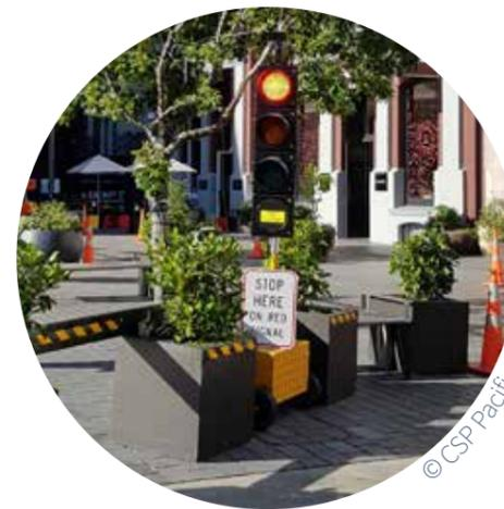
Trailer mounted portable traffic lights (PTL) for an interim event can be used to temporarily control an intersection and measure light timing and phasing.
